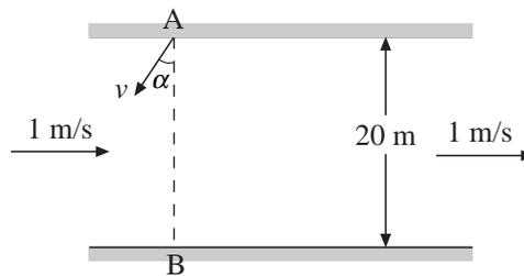
A river is flowing steadily at a speed of 1 m/s. A motor boat leaves point A on one side of the river. The boat has a constant speed,  $v = 2$  m/s.
