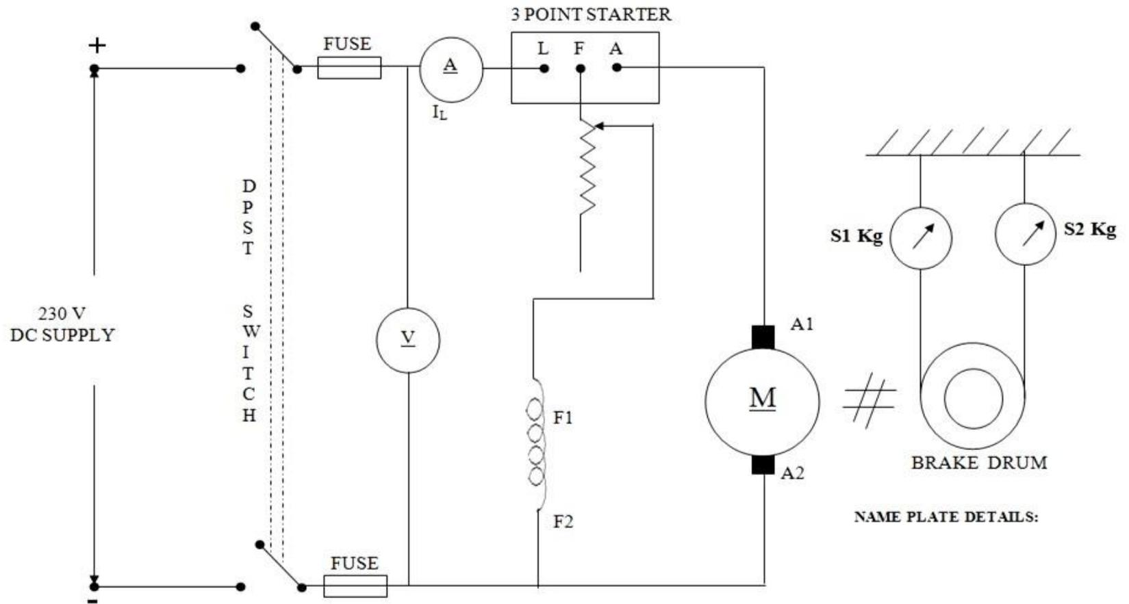
Figure 1.1 - Load Test on DC Shunt Motor
